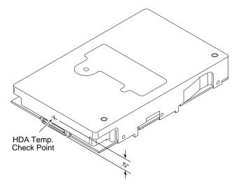
Figure 9. HDA case temperature measurement location
