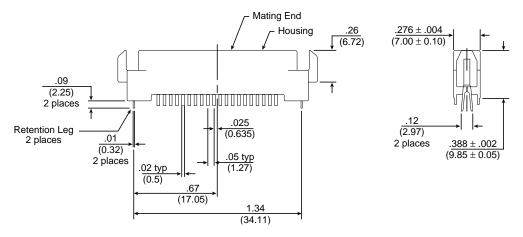
Figure 12. FC-AL SCA device connector dimensions
