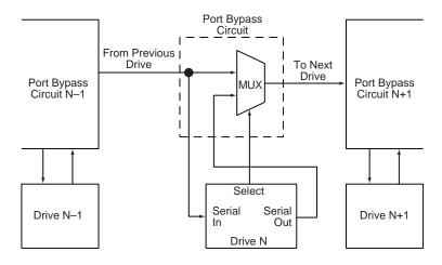
Figure 11. Port bypass circuit physical interconnect
