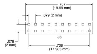
Figure 13. J6 connector dimensions
