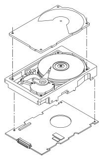
Figure 2. Cheetah 4LP FC disc drive
