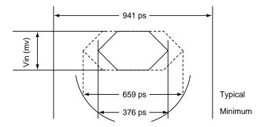
Figure 16. Receive eye diagram
