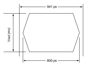
Figure 15. Transmit eye diagram
