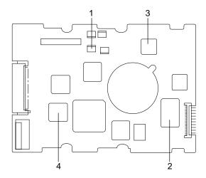
Figure 8. PCB temperature measurement locations
